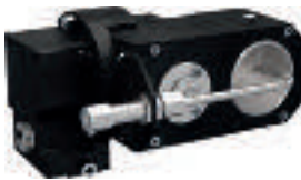
■ Thread whirling unit max. 5700 min -1 angle +/- 15° Ø max. 10 mm
